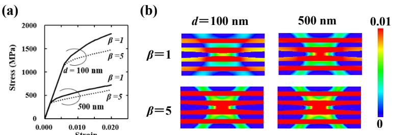
Fig. 2 (a) Stress-strain curves of ferrite phase with different layer thicknesses  $d$  and dislocation absorption abilities  $\beta$  and (b) distributions of equivalent plastic strain in  $(\theta/\alpha/\theta/\alpha/\theta/\alpha/\theta/\alpha/\theta/\alpha/\theta)$  lamellar structures when tensile strain is 1.7 %.
